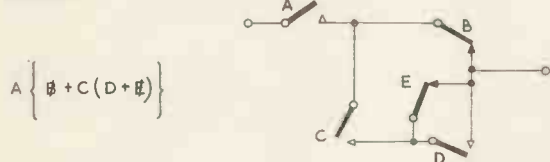
Fig. 2. Boolean algebra applied to switching circuits
