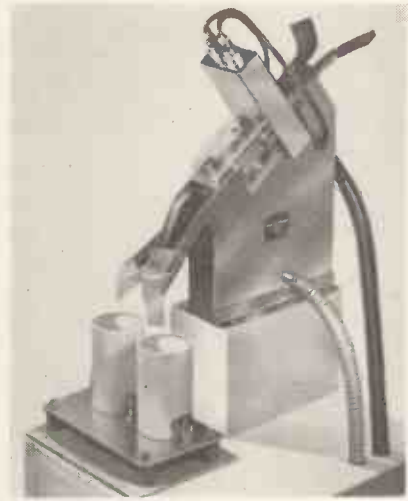
Fig. 5. Dual batching mechanism consisting of twin optical system and ganged high speed batching gates for alternate filling of cartons
