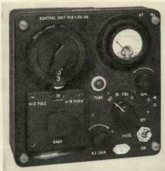
Fig. 1. STR.18C 100 channel pilot's remote control unit
