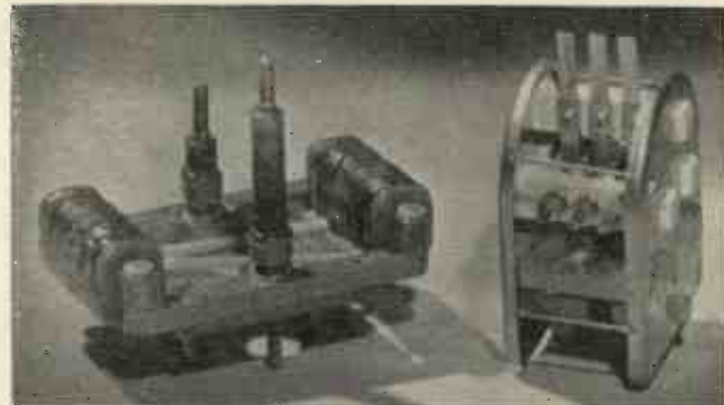
Fig. 3. The external magnetic circuit of the relay showing its connexion to the two threaded pillars which are normally sealed in the glass base and connect with internal magnetic circuits, armature and contact assembly shown on the right
