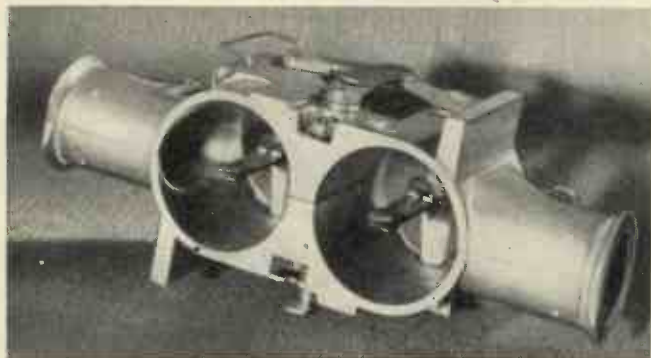
Fig. 12. Switch-unit of twin coaxial commutator
