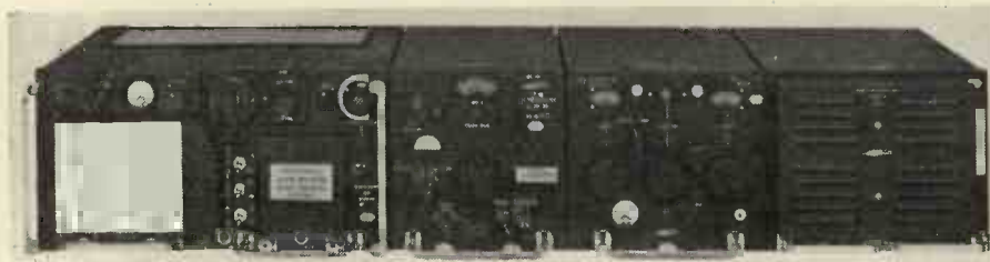
Fig. 2. STR 18C 100-channel H.F. airborne communication equipment
