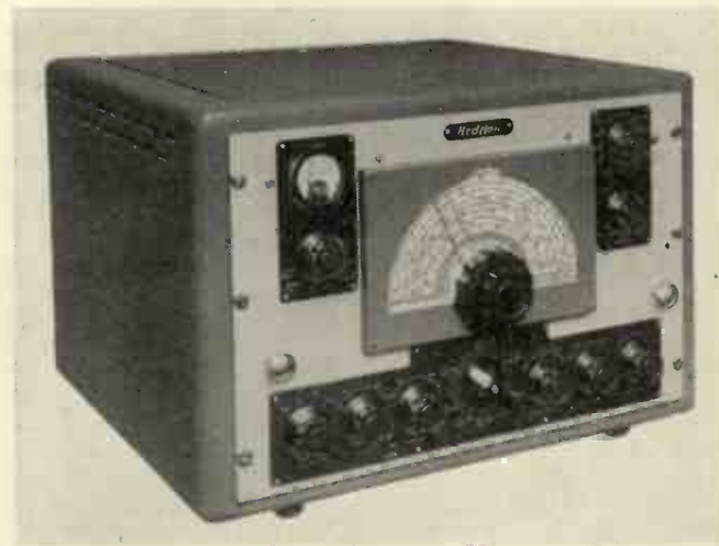
An approved receiver for compulsorily fitted ships (Redifon type R50H)
