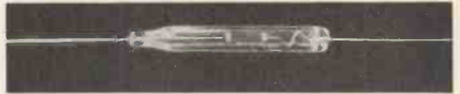
Fig. 5. Megistors. High value resistors in range 10^7 to 10^{13} ohms. (Courtesy of Morgan Crucible Co. Ltd.)
