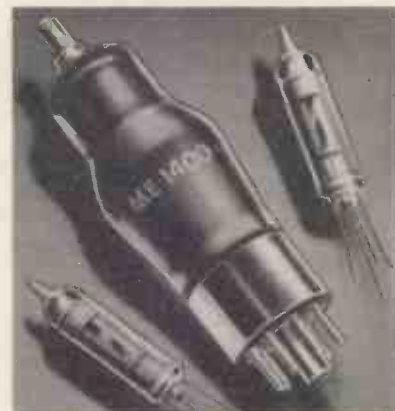
Fig. 6. Electrometer valve types ME1400 and sub-miniature models ME1401 and ME1402
