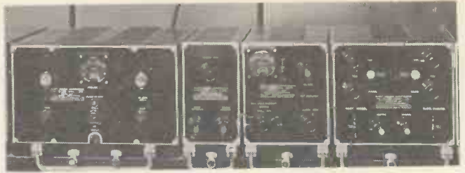
Fig. 3. An airborne magnetometer instrument built on standard S.B.A.C. racking
