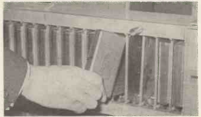
Fig. 9. Sealed and oil-filled printed circuit units 5in x 3in, and rack with water-filled cooling baffles in which they are placed The baffles have flexible sides which form good thermal contact with the unit when hydrostatic pressure is applied.
