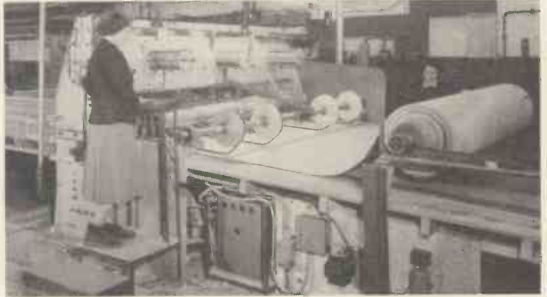
Fig. 5. Length measurement of veneer
