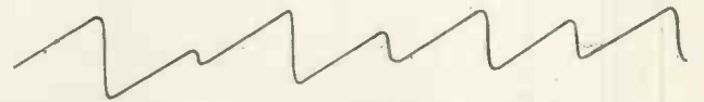
Fig. 5. Starting conditions of deflector-coil current which will occur in circuits of the type shown in Fig. 4. Double stroking occurs, but the waveform eventually settles down
