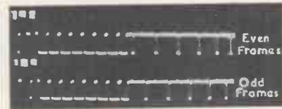
Fig. 4. Oscilloscope obtained using 50c/s scan and 25c/s square wave to separate the two frame waveforms. Positive picture signal from pattern generator
