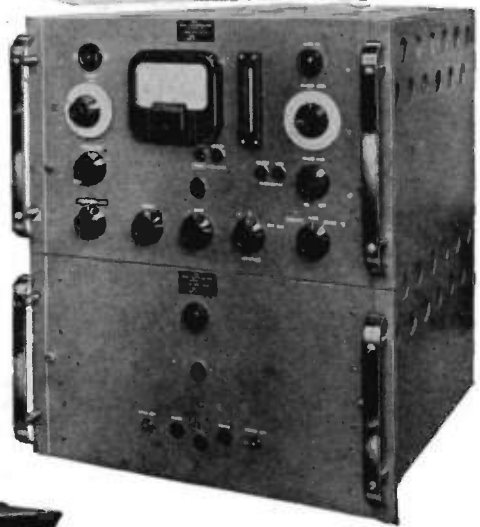
▲ Type FSK.2. Keying Unit for frequency-shift keying is designed for conversion of any conventional communications transmitter for frequency-shift operation.
