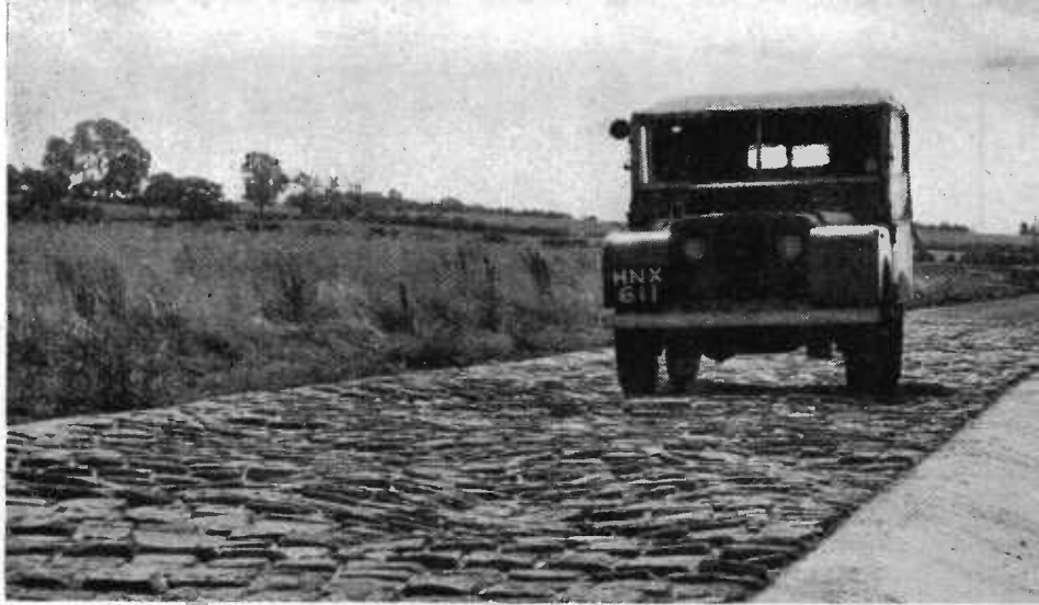
A vehicle being subjected to endurance tests on a section of Belgian pavé surface at the M.I.R.A. Proving Ground.
