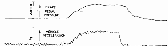
Fig. 5(b). Typical record of brake pedal pressure and vehicle deceleration obtained with equipment shown in Fig. 5(a)
