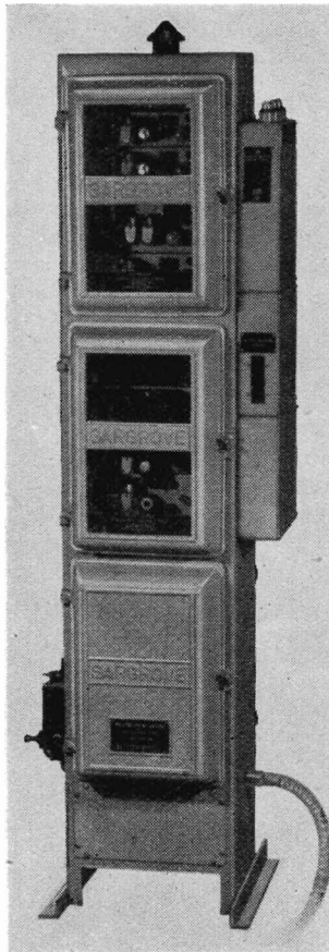
The control cubicle containing the electronic control apparatus of the extrusion plant and electronic micrometer.
