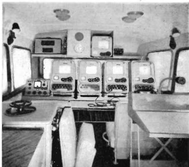
An interior view of one of the television outside broadcasting vehicles. Left to right (foreground), store cupboards, power regulating unit (main desk broadcast distribution box, three camera control monitors, master control monitor and mixing. (Above) sound receiver and "on the air" vision receiver. (Extreme right) producer's desk.
