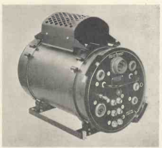
The cylindrical type of sealed radar unit, one of the first of its kind to be developed. This is part of Rebecca Mk. IV, reproduced by courtesy of Messrs. E.M.I. Factories, Ltd.
