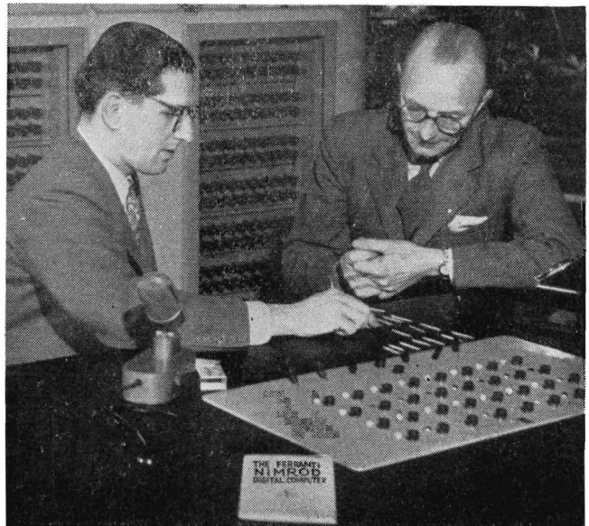
The control desk of Nimrod. The players are studying the game by using matches in addition to the push-buttons and lights.
