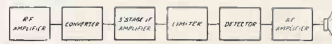
Fig. 1. Block diagram of a receiver designed for the reception of frequency-modulated signals. With the exception of the limiter stage, the lineup is similar to that of a conventional superheterodyne receiver.
