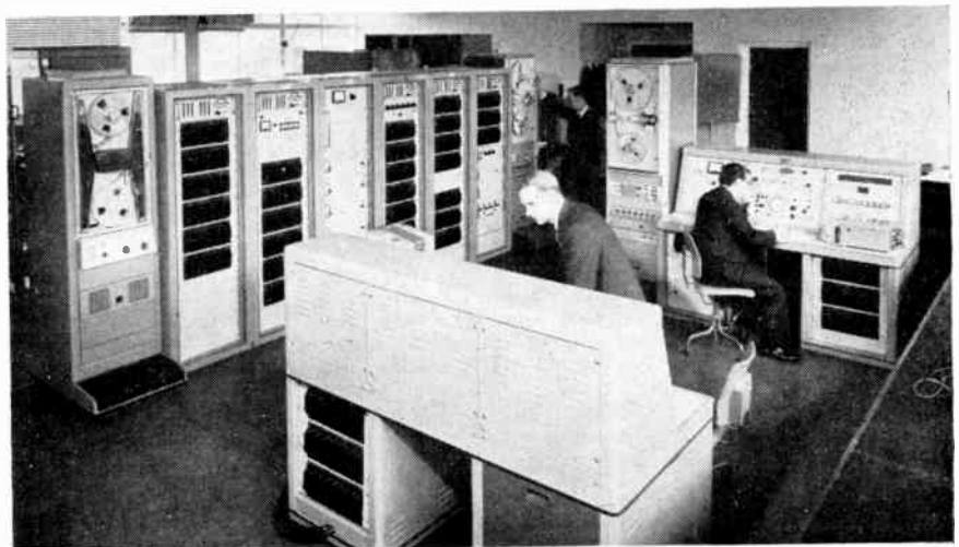
General view of the data processing equipment at the Radio Research Station, Slough. The control console is seen in the foreground and to the right is the tape editing console
