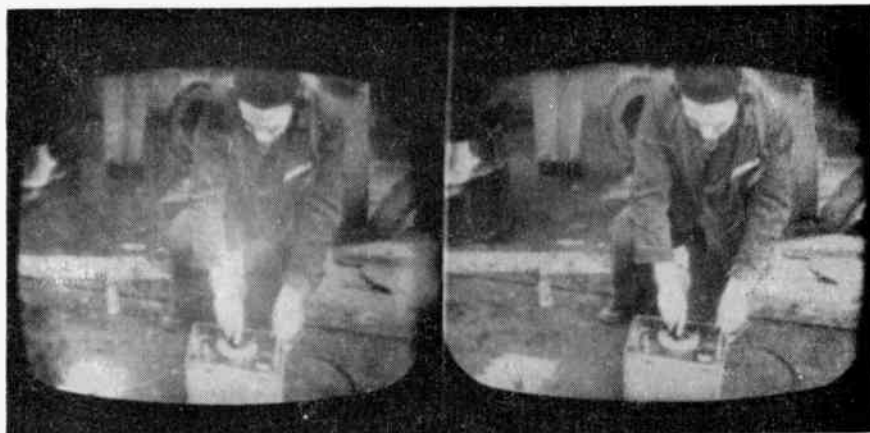
Fig. 8 (right). Picture from monitor connected direct to television camera. (left) Picture from monitor carrying read-out stored picture, 5 minutes after receiving one field from camera (Note central area fading white due to discharging effect of positive ions)
