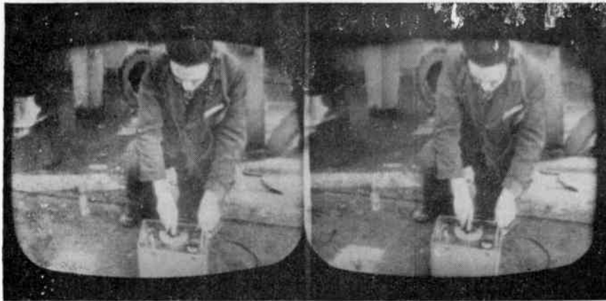
Fig. 7. Picture storage: (right) Picture from monitor connected direct to television camera. (left) Picture from monitor carrying read-out stored picture, one minute after receiving one field from camera
