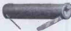
Type 36EHT rectifier. Two such units only 2\frac{1}{2} " long by \frac{3}{8} " dia. will give an output of 5.3 KV.
