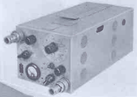
Above: Lightweight M.F. broadcast receiver with simple D.F. facilities. Left: 5-channel V.H.F. transmitter-receiver, type TR.51, for light aircraft
