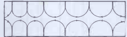
Fig. 5. E_{010} resonator suitable for electron acceleration
