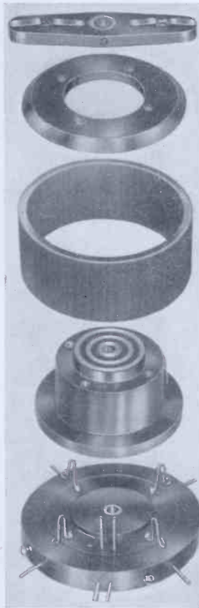
Fig. 4. Exploded view showing construction of special toroidal potentiometer. The wound ring fits over a moulded baseplate in which are four symmetrically placed contact springs to give tappings at 90°. The current is fed to the winding by the rotating arm (top) in which two silver pins make contact with the winding and two concentric sliprings. The main shaft is not shown in the photograph.
