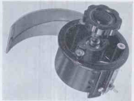
Fig. 3. Left: Potentiometer with special "cam correction" device
