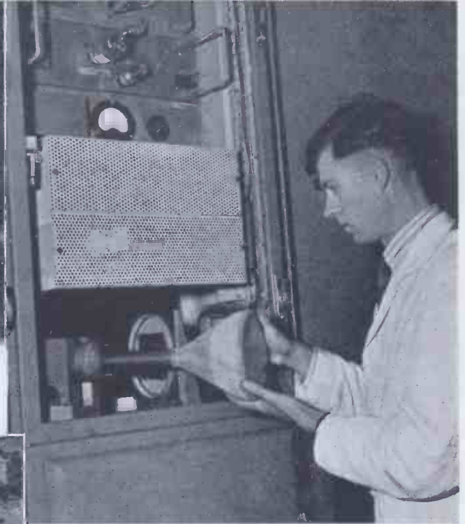
The Emiscope projector tube being fitted to the E.M.I. film scanner. The 9" tube has an optically flat screen and is operated at 15 KV.
