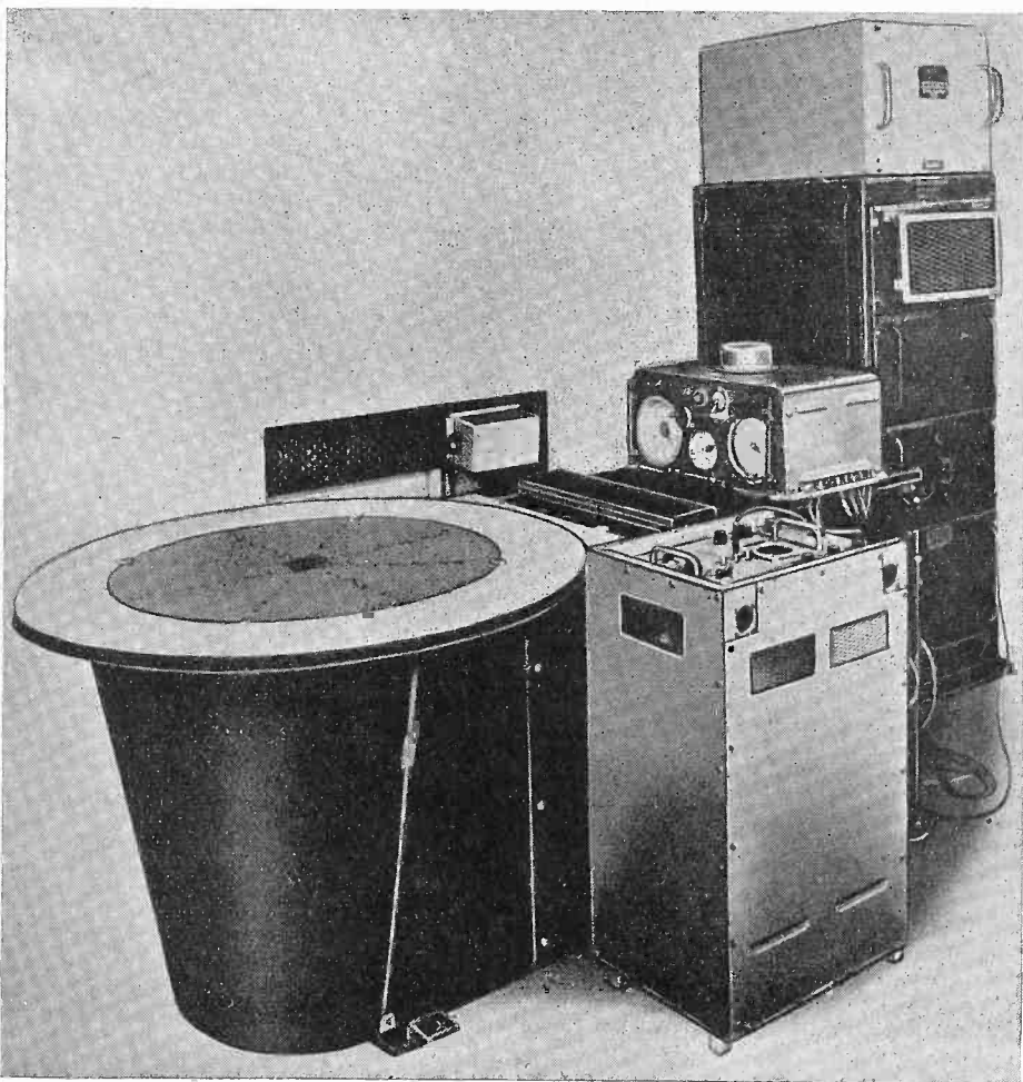
Fig. 4. Screen of the plan position indicator with dark trace tube
