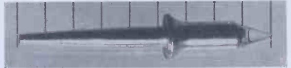
Fig. 8. Enlarged view of needle, showing collar and sapphire tip. (Scale marking in mm.)
