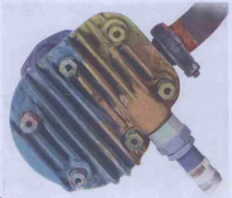
Fig. 3. (above). Air-cooled cylinder showing temperature rise around valves.
