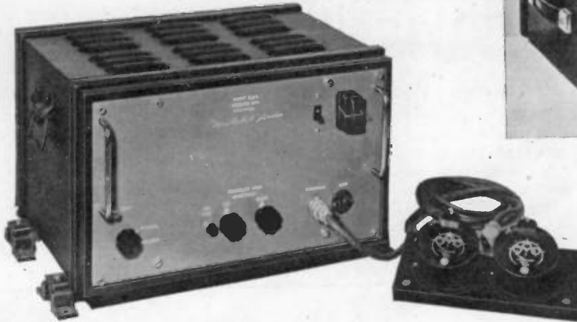
Fig. 9. Battery-driven portable receiver, showing control panel. The dials are viewed through the circular windows on top.
