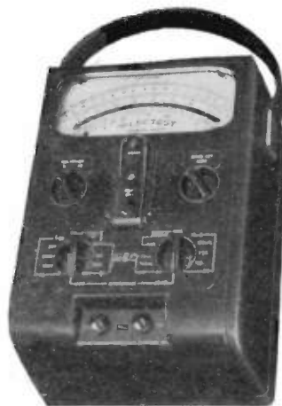
Multi-range A.C. D.C. testmeter. 1,000 \Omega /V with safety and overload devices.
