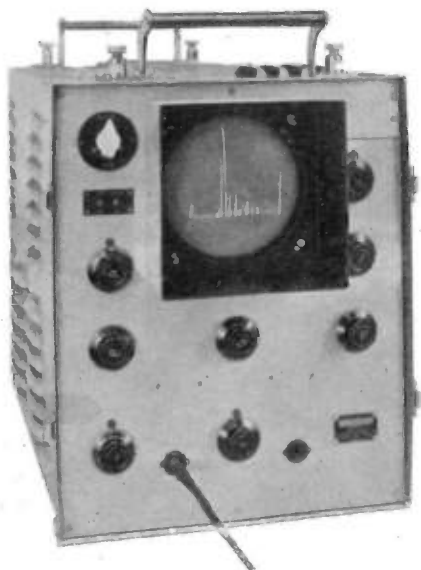
(Left): Frequency spectrometer giving individual components of a complex waveform. 40-16,000 c/s. or 8 kc/s.-3,200 kc/s.
