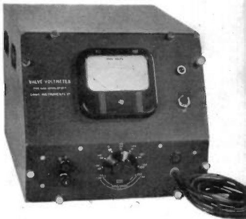
(Below): Sensitive valve voltmeter with feedback amplifier. Range, 0.03-300 V in 9 steps. Frequency response linear from 10 c/s. to 1 Mc/s.
