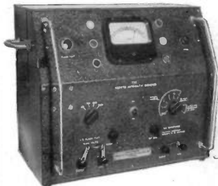
Automatic ohmmeter manufactured by the Mervyn Sound & Vision Co., Ltd. This automatically selects the optimum range for the resistance under test to give a reading on the most accurate part of the meter scale. Range, 1 \Omega -10 M \Omega .
