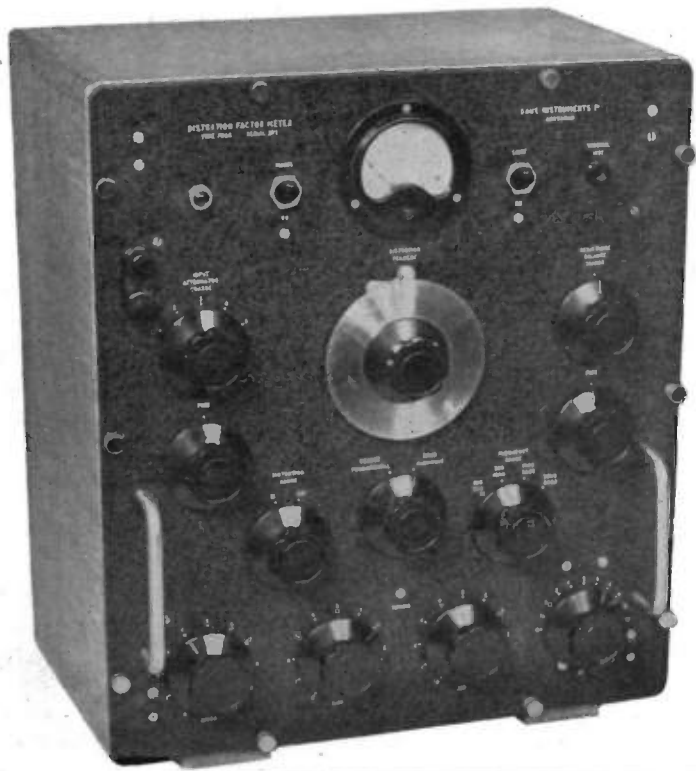
(Below): Distortion factor meter for measuring total harmonic content of A.F. apparatus.
