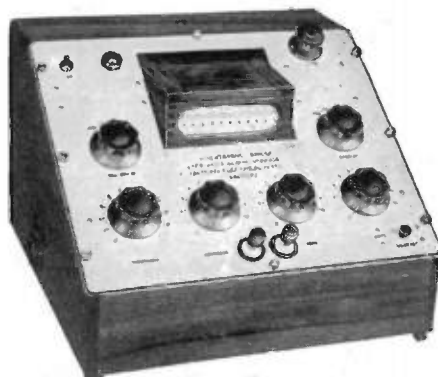
Wheatstone bridge of new design with built-in A.C. supply and galvanometer. Range, 0.1 \Omega -10 M \Omega .
