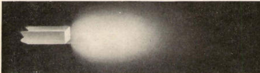
Distribution of light as above but with the output end lightly roughened by sandpaper.
