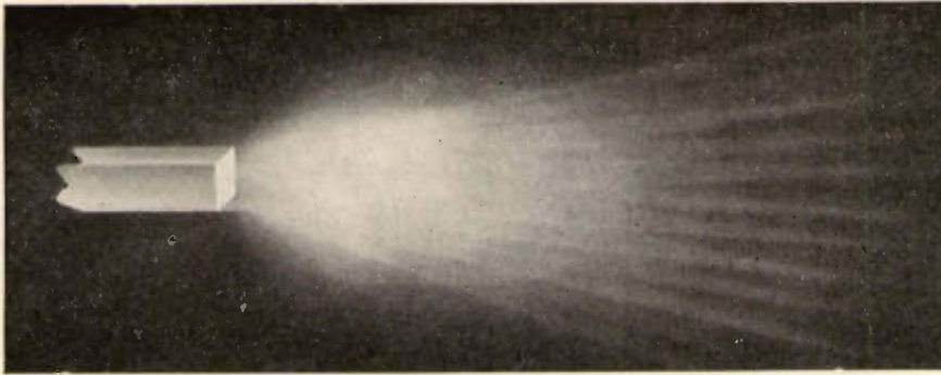
Distribution of light at end of a 10-inch Perspex rod with the lamp 1 inch from other end. Ends of rod polished.
