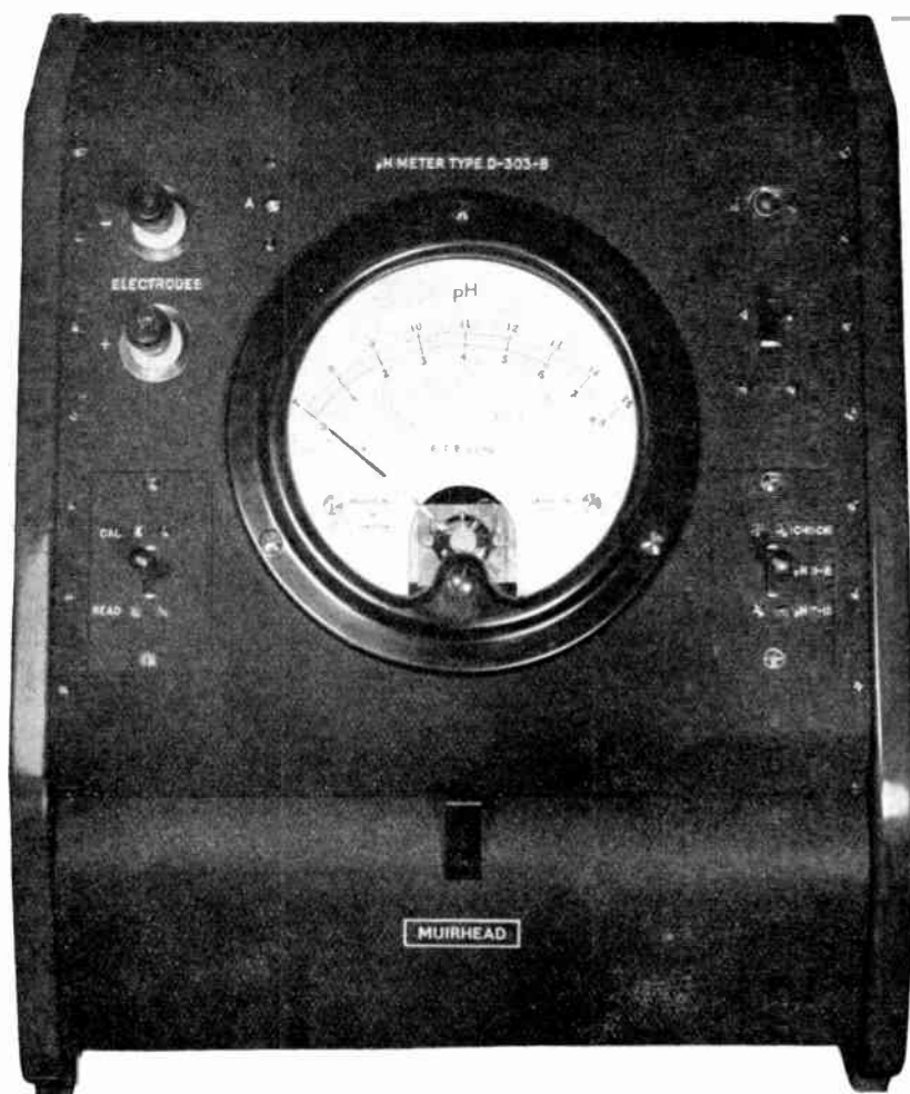
General view of pH meter.
