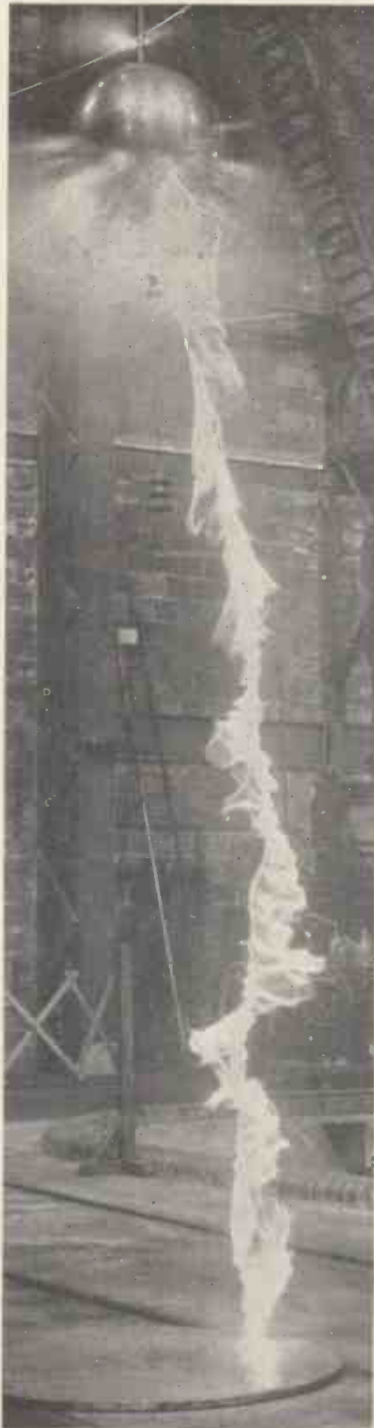
Artificial lightning (a one million volt flash). Taken at the Research Lab. of Metropolitan Vickers Electrical Co. Ltd.
