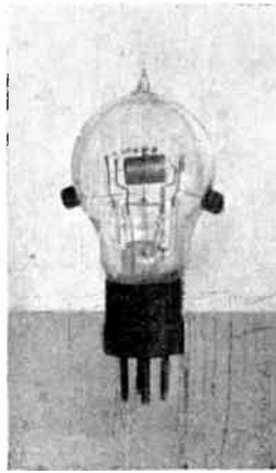
Early low-capacity triode—the "horned valve,"
