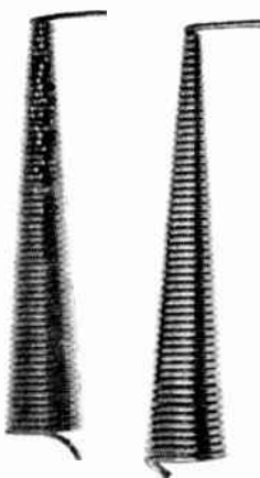
Thermex wire (right) and enamelled wire after 150° C. heat shock.
