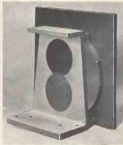
Close-up of lens mounting showing filter disks in front of each lens.
