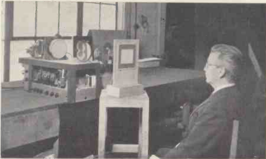
Photograph of experimental apparatus for showing coloured pictures with two-colour filter disks
