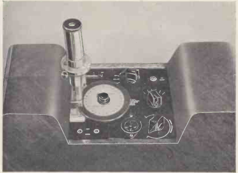
View of top panel of Electrocardiograph, showing recording disk and microscope in place. The patient leads are plugged into the sockets near the front edge.
