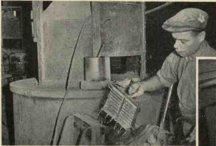
Casting lead grids in pairs for the battery plates.
