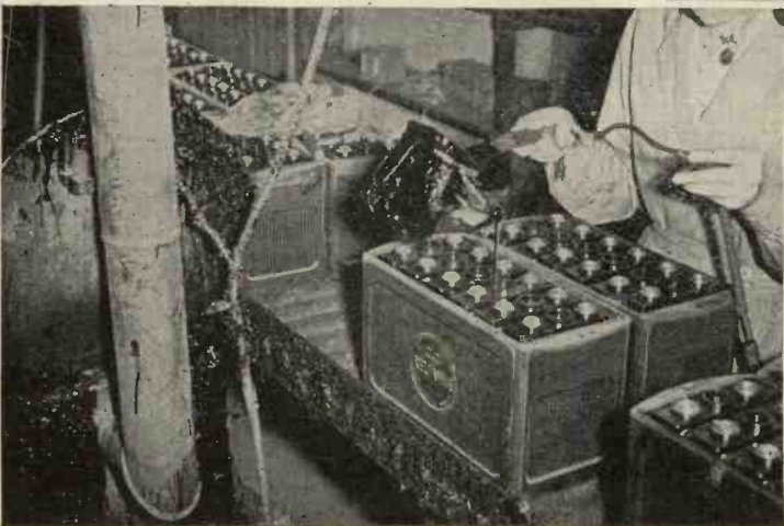
(Above) Fitting wood separators between plates. (Left) Sealing in tops of finished batteries with compound.
