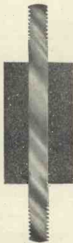
A copper insert has become an integral part of the whole through close adherence to the MYCALEX surround.
