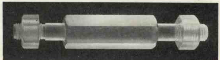
Bolt and nut machined from Distrene. This specimen is intended to show the ease with which the material can be worked by the usual mechanical processes. There is no tendency to chipping on the edge of the thread. Messrs. B.X. Plastics
