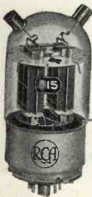
Fig. 18. The R.C.A. 815 push-pull beam tetrode, having a max. total anode dissipation of 25 watts for ICAS service at an anode voltage of 500. Ratings are 100 per cent. down to 300 cm. Bulb diameter 2".
