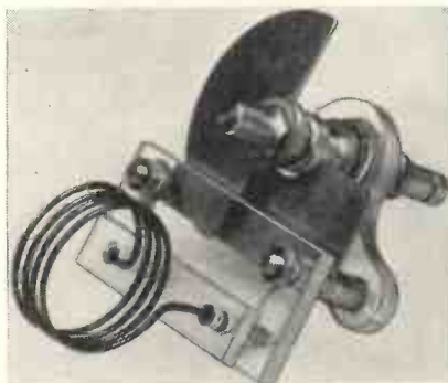
This is the plug-in 5-metre coil in the 6L6G anode circuit.
