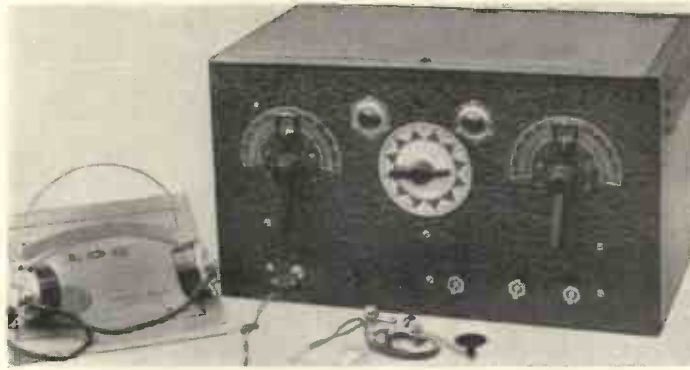
This front view gives a good idea of the controls and layout. The transmitter is designed for C.W. operation and cathode keying.
