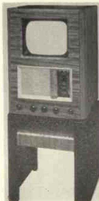
Left: Baird table model T20 giving a picture 10 ins. by 8 ins.
