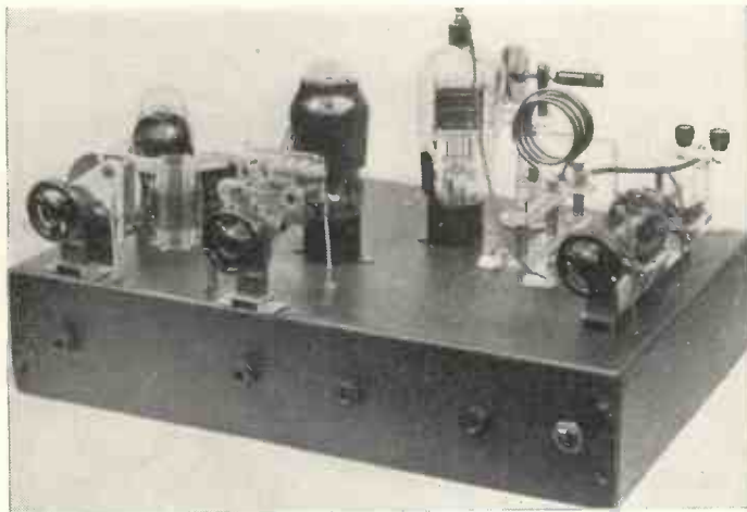
Two wide-gap midget condensers are used as a split stator in the final stage.
