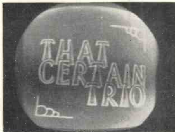
Fig. 11. Here, the presence of hum in the receiver output results in the production of a dark horizontal band across the picture. The position of this band will depend upon the relationship existing between the supply mains.
