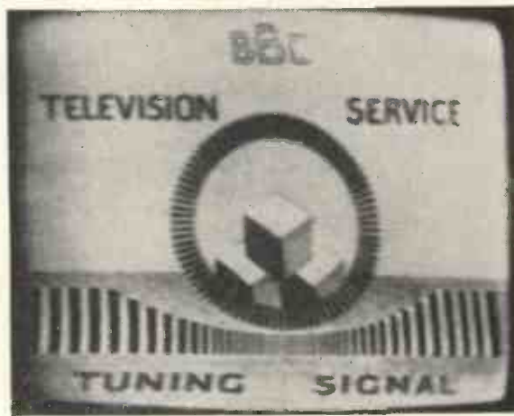
Fig. 3. In this photograph the line synchronism is well maintained during the framing period as is revealed by the steadiness of the upper portion of the caption. The slight-off vertical inclination of the lettering is due to bulb curvature.
