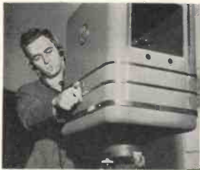
General Electric's television camera. The small, circular holes contain red lights which glow, signalling the actors when the camera is in operation.
