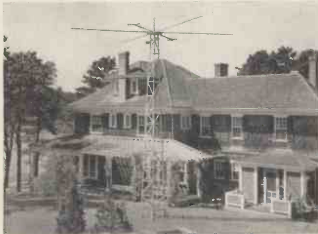
This is the half-wave rotary aerial in use at W1KKP. Its effectiveness is proved by the fact that this station can often be heard when the 20-metre band is quite dead for long distance reception.
