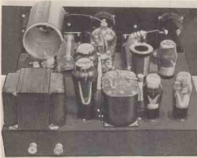
Two special transformers are required in the speech amplifier which consists of two 6L6's in class-A push-pull.
