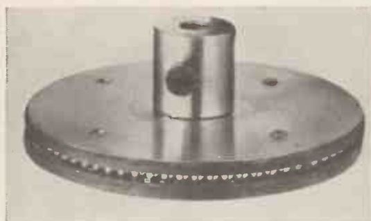
Above is a photograph of the high-speed scanner, which consists of a series of steel balls held between two brass discs.
