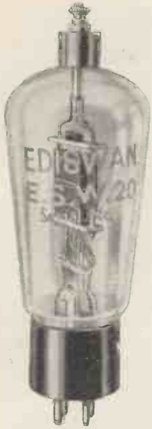
This Ediswan triode the ESW-20 is of the low capacity type suitable for high-frequency operation.
