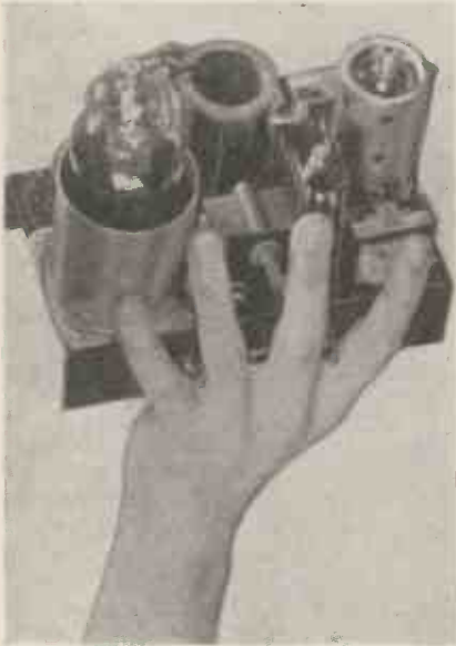
This close-up view very clearly shows the tuning condenser, microphone transformer and both 802 and 89 valves.
