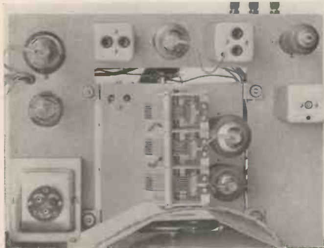
This plan view shows the complete tuner and the layout of the other components. The trimmers in the I.F. transformers are adjusted by the manufacturers and should not need further adjustment.
