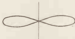
Fig. 4b. Effect of splitting aerial of Fig. 3a and feeding each half in phase.
