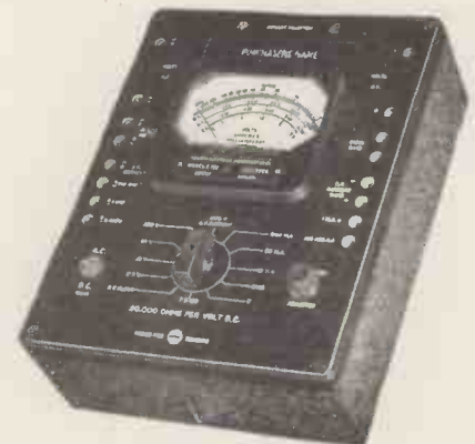
Fig. 5.—The Weston service analyser.
