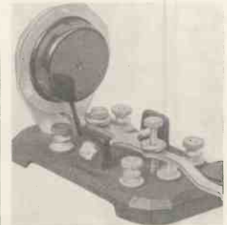
A key plus hummer of this type is very helpful for the beginner for the hummer produces a note similar to the morse code heard on a radio set.
