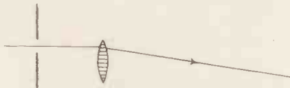
Fig. 2.—Showing the deviation of a ray at different points on the lens surface.
