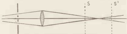
Fig. 4.—Chromatic aberration demonstrated by placing the ground-glass screen at S or S' the coloration of the edges of the images of the slits (outer edges red at S, blue at S') is shown.
