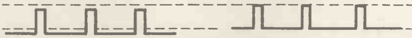
Fig. 3. The signal given by a blank line, showing how the mean potential across a condenser rises until equal areas are obtained on each side of the line.
