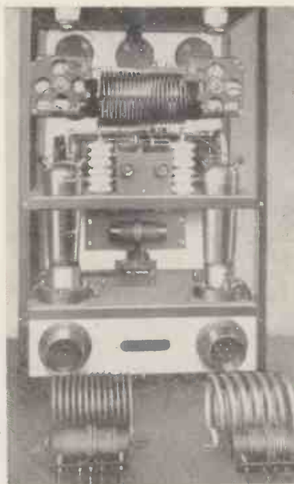
The R.F. amplifier section is very well built and carefully screened in order to obtain straightforward operation on three wavebands.
