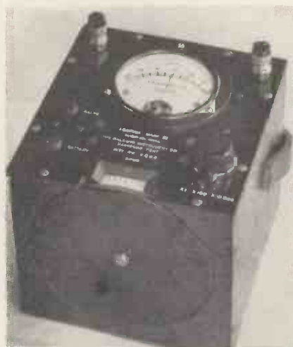
Fig. 4.—The Baldwin resistance bridge: note the neat dial arrangement.
