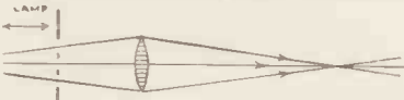
Fig. 3.—Divergent pencils: By sliding the lamp to and fro the variation of the focus with variation of object distance can be seen.
