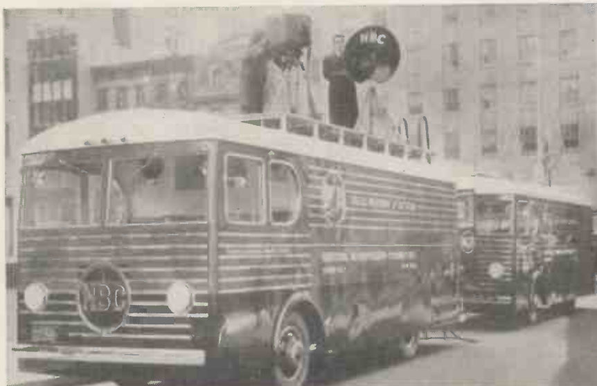
America's first mobile television station, to be used by N.B.C. engineers in experimental pick-ups of outdoor news events, is shown as it was delivered to the National Broadcasting Company at Radio City.
