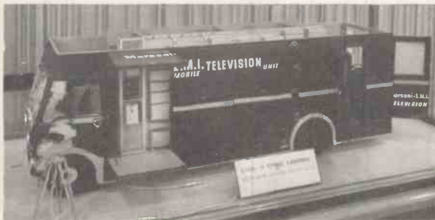
A scale model of the Marconi-E.M.I. mobile equipment for outside television broadcasts. At the left is the Emitron camera.
