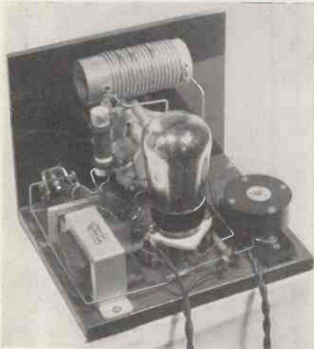
In this transmitter the coil is mounted on the panel but gapped about half-an-inch with two small pillars. Similarly with the valveholder, which is of the ceramic chassis type, this is mounted off the baseplate on two stand-off insulators. The crystal, seen on the right-hand side, should be of the wavelength on which the operator intends to work.
