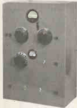
10 watt A.C./D.C. C.W. Transmitter. Pentode Crystal Oscillator. Low crystal current. Minimum frequency drift. Price complete with Valves, Crystal and Key, £4 4s.
