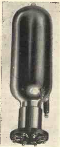
Baird Multiplier photo-cell type ML.
