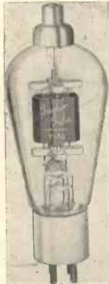
This is the Taylor T-555 carbon anode triode for R.F. or audio work. As an audio amplifier the output for two values is 250 watts with 1,500 volts H.T.
