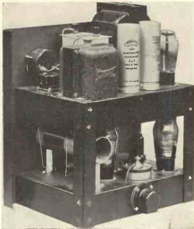
The transmitter, single speech amplifier and modulator are all housed in the bottom rack with the power pack and modulation transformer in the top rack. The two chassis are interconnected by means of 5-way cable.
