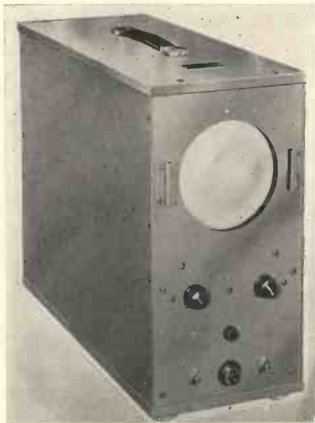
The Cossor model 3313 high-vacuum tube unit.
