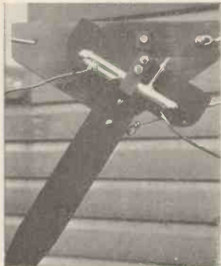
The glass tube is mounted on a T-square in the exact centre of the aerial. Platinum contacts must be used.
