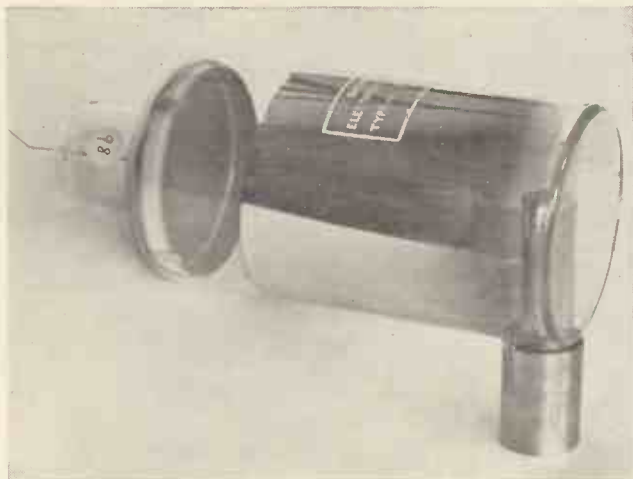
The tube in which the electron image is formed and scanned in the manner described in the text.
