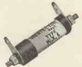
Westectors. Suitable for detection and/or A.V.C.
