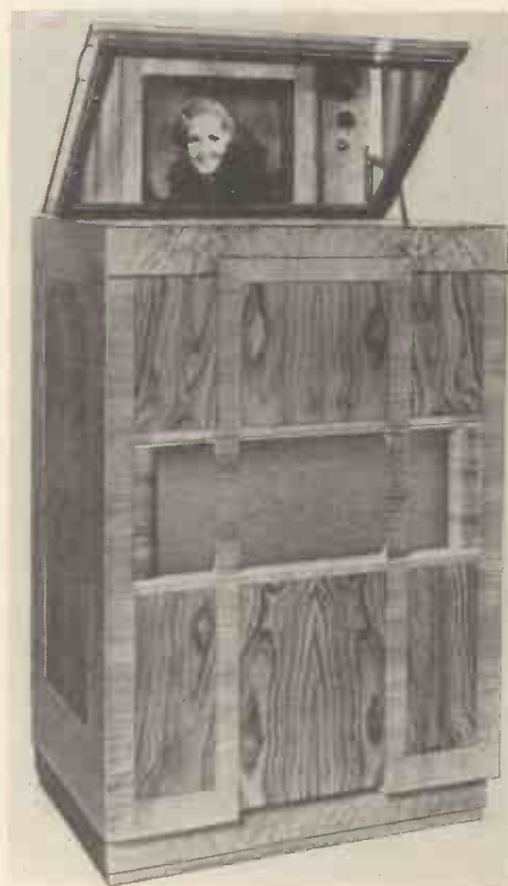
The photograph on the left shows the Marconiphone television receiver capable of receiving the Alexandra Palace sound and vision transmissions and also all broadcast sound. Model 702 (right) is for television and accompanying sound reception only.
