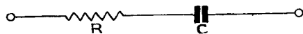
Fig. 21.—The form of impedance arm which should be substituted for R in Fig. 16a to provide correction at low frequencies.
