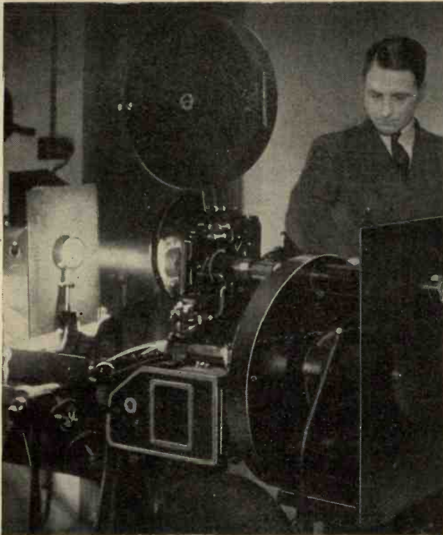
The Baird high-definition Telecine transmitter.
