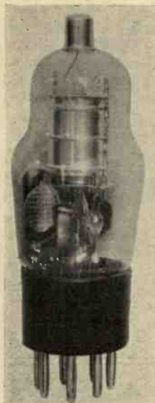
This is the X41 triode hexode with a 4-volt heater. It is also available in the universal range and is designated the X31. Although primarily intended for normal short-wave working it proves excellent down to four metres provided the circuit on this page is used. Make sure to screen the grid from the oscillator so that the only coupling is via the electron screen.
