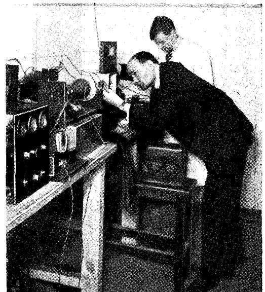
Use of the cathode-ray tube for recording pictures on film for television reproduction in cinemas.
