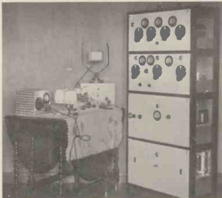
The top rack houses the push-pull oscillators, while in the second rack are a crystal oscillator, frequency doubler, and link-coupled buffer. Ten valves are used in the speech amplifier—modulator—power pack in the third rack, while four valves are used in the bottom rack for the two power packs.
