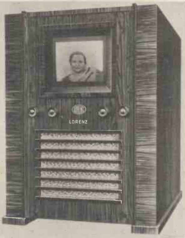
A view of the Lorenz television receiver with a tube by Manfred von Ardenne showing an actual television picture.
