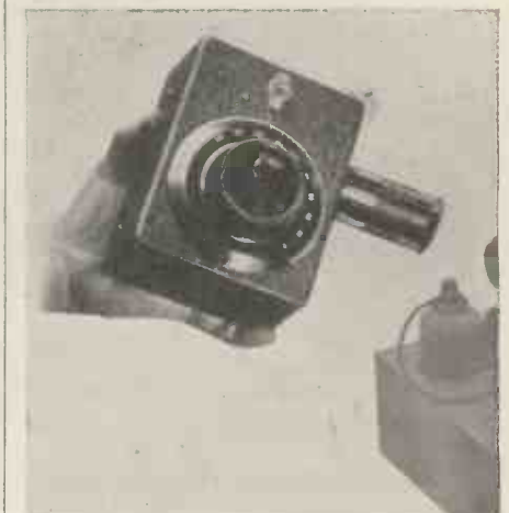
This wavemeter is a combination buzzer-absorption. It is selective and will tune down to 9.5 metres.
