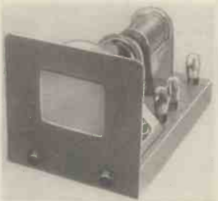
This photograph shows the cathode-ray tube chassis and screen.
