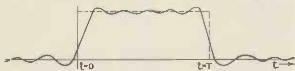
Fig. 16. (left)—Effect of high-frequency cut-off on a square-topped wave.
