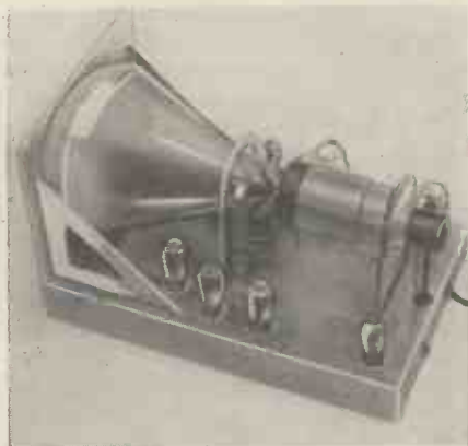
A side view of the cathode-ray tube with deflector magnet and deflector coil in position.
