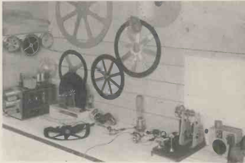
A corner of the test bench showing various types of scanner. Note the perfectly flexible disc in the foreground used for experimental work. View includes a standard 60f-disc set and Diosphere mirror drum unit.
