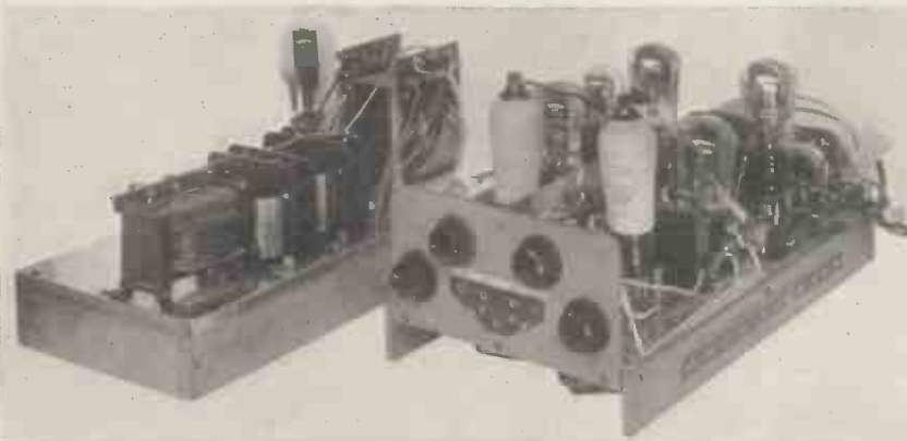
A close-up view of the time base and exciter units. Note the extra smoothing chokes on the H.T. units.
