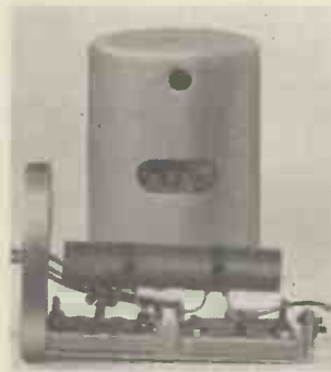
Fig. 2.—The B.T.S. I.F. transformer.
