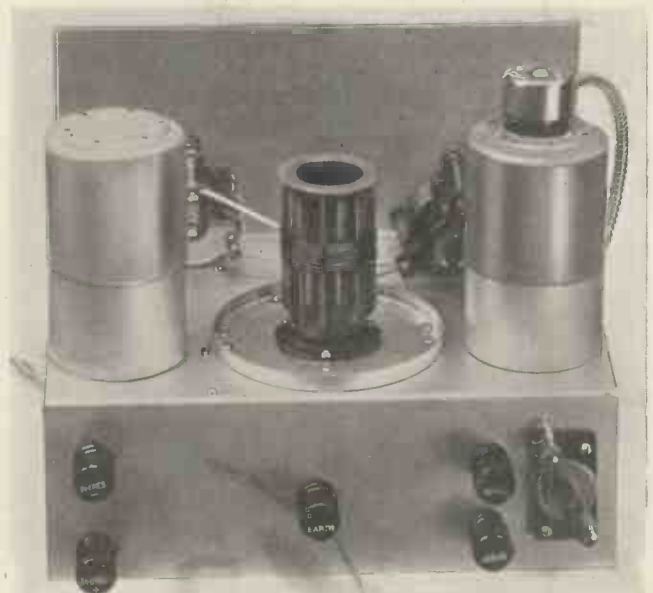
An aerial preset condenser is fitted to the back of the chassis. It can be cut out of circuit by using the alternative aerial connection.
