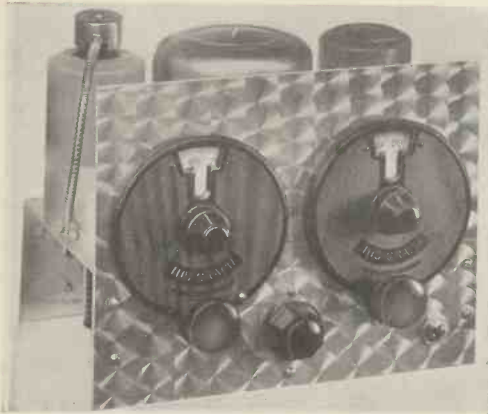
The left-hand control is the master tuner, the dial on the right being for band spread.
