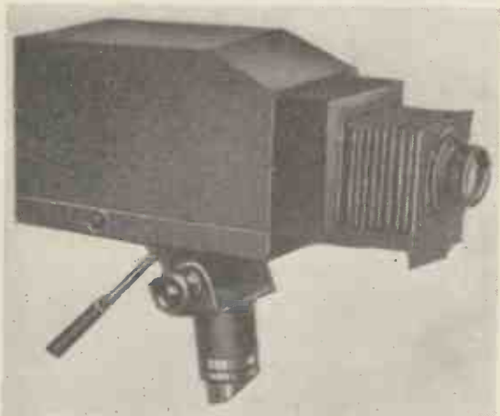
The dissector-multiplier camera for direct electronic scanning. (From the Journal of the Franklin Institute.)
