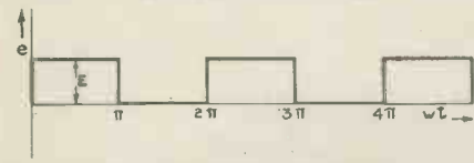
Fig. 2.—A periodic D.C. impulse which can be represented by the series for Fig. 1, plus a constant term.
