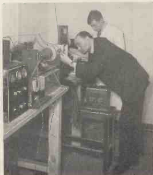
Using a cathode-ray tube for recording pictures on film for television reproduction in cinemas.
