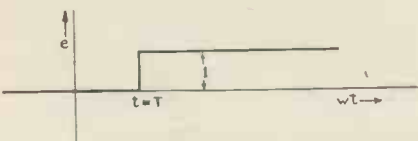
Fig. 5.—A unit amplitude D.C. wave taking place at time t = T .
