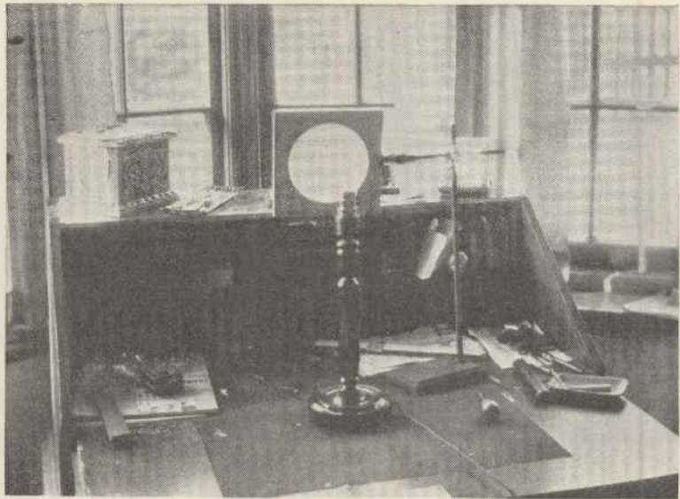
Fig. 6.—A grease-spot photometer is very easily set up as this photograph shows.
