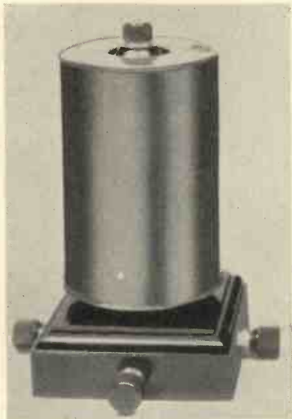
The photo-cell mounted in its screening can.
