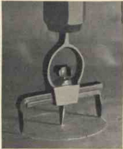
Photograph showing how the holes are cut.
