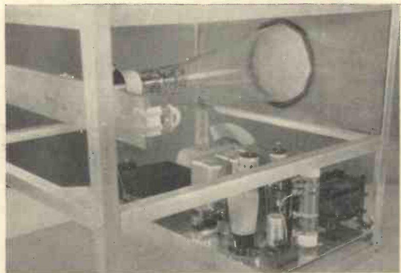
This photograph shows clearly the method of supporting the rear end of the cathode-ray tube.
