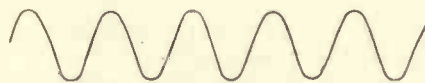
Fig. 4. The appearance of the trace when there are stray magnetic fields present and the 375-cycle base is cut off.
