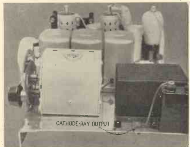
This photograph shows the two output terminals for the cathode-ray tube.
