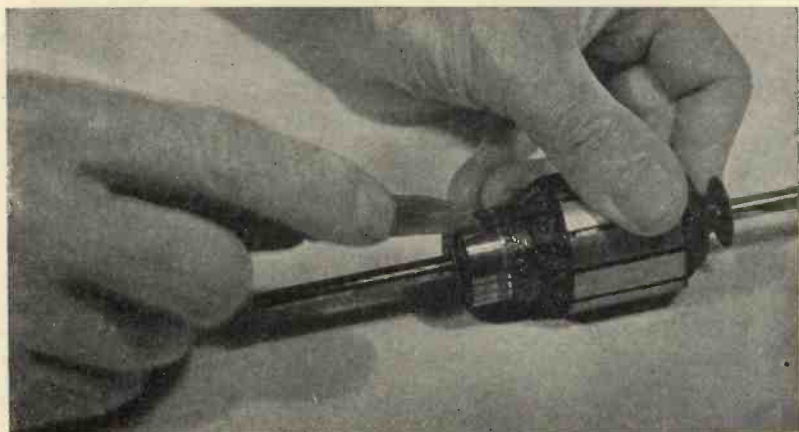
Sparkling is frequently due to high insulation between the commutator segments: this photograph shows how it can be reduced.
