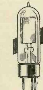
A neon lamp of the flat-plate type.
