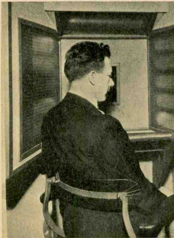
In this kiosk used at the Bell Laboratories, the photo-electric cells can be seen behind the glass plates surrounding the sitter.
