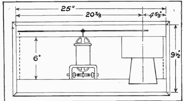
Fig. 4.—A plan of the baseboard lay-out supported on the plinth.
