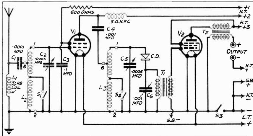
Fig. 1.—Complete details of the theoretical circuit drawn up by Mr. William J. Richardson in the design of the "Crystal" Three.
