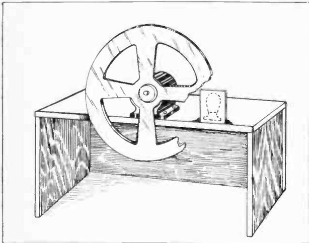
Fig. 1.—Testing discs by the use of a ground-glass screen secured by plasticine, the neon lamp being replaced by an ordinary filament lamp.
