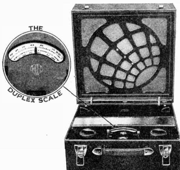
Showing the McMichael Duplex Four portable receiver. The pointer moves to the appropriate scale as the waveband switch is operated.
