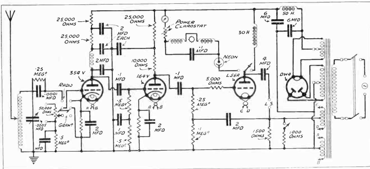
Messrs. E. J. and J. W. Holmes carried out a large number of experiments before deciding on their final vision wireless receiver circuit. The complete scheme is shown in the diagram above.
