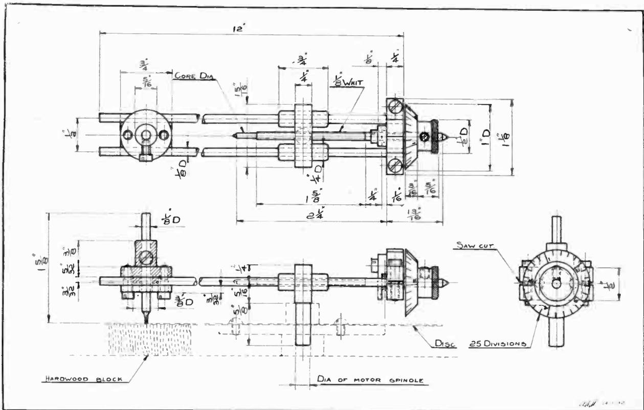
The complete working drawings of the trammel designed by Mr. R. W. Martin.
