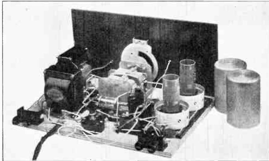
does normal service for this purpose. Depending upon what type of neon is used in the vision apparatus, so the voltage and current of the H.T. + connection will vary. My own tests were carried out with a Baird "Televisor," and the voltage of 200, giving a current of 25 milliamperes, suited admirably.
