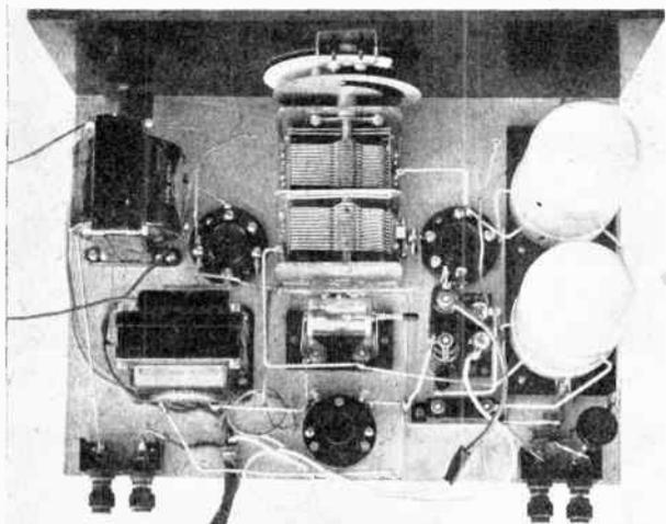
A good plan view of the completed receiver which can be compared with the wiring diagram of Fig. 3.
