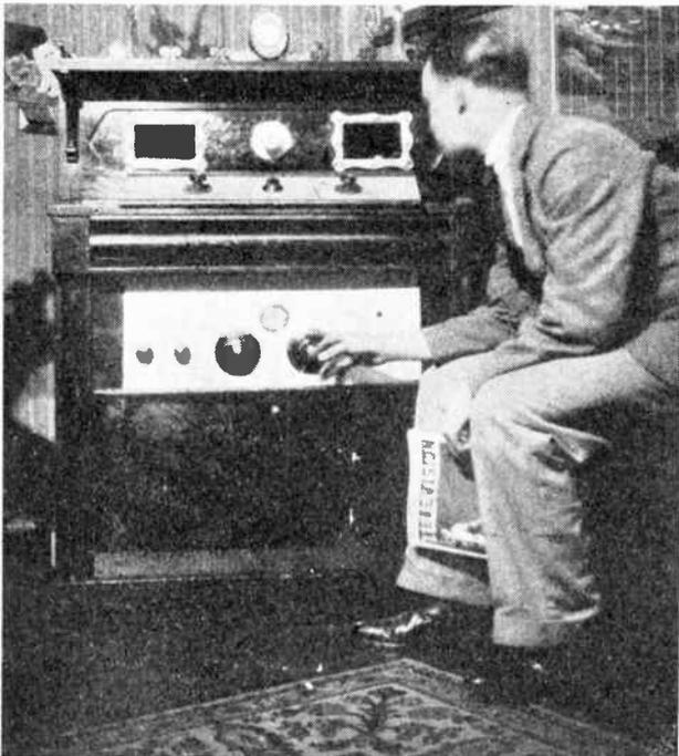
*Another amateur version of a dual vision and sound wireless receiver built into a cabinet complete with loud speaker and vision apparatus.*
