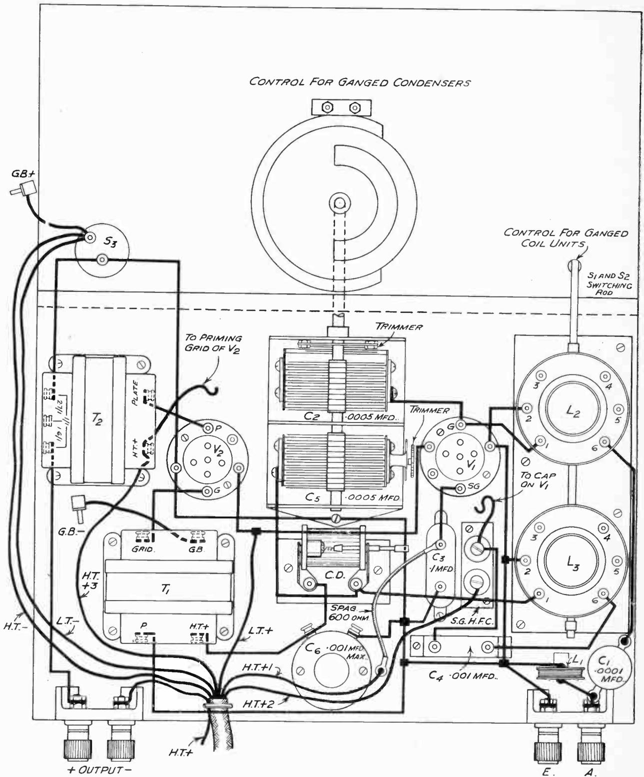
Fig. 3.—A true-to-scale reduction of the original wiring diagram for the back of panel and baseboard. Make all your own connections in the manner shown, using the photographs to enable you to visualise "wiring runs."
