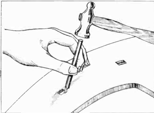
Fig. 2.—Correcting white lines on a disc by "closing" the hole with a light tap on a punch.
