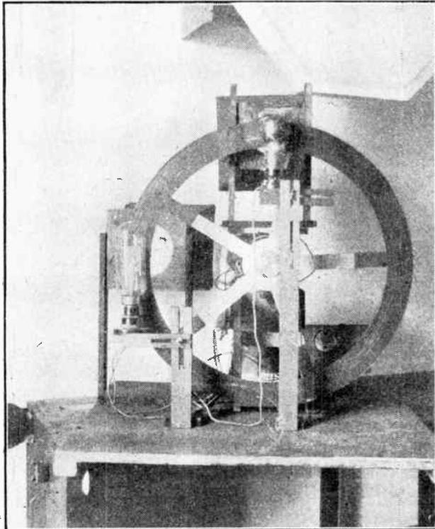
*Looking at the back of Mr. Foster Cooper's vision apparatus. Both vertical and horizontal scanning may be employed, the separate neons for this purpose being clearly visible.*
