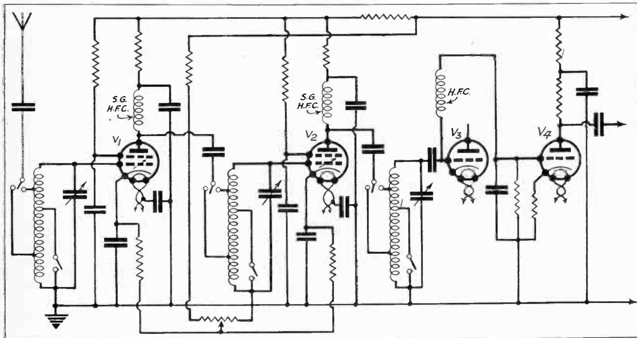
Fig. 1.—Mr. Barton Chapple's suggested scheme for the high-frequency and detector stages of the Tele-Radio Receiver. Volume control is secured through the medium of variable-mu valves, while a diode valve is to be employed to rectify the signals before they pass to the low-frequency amplifier.
