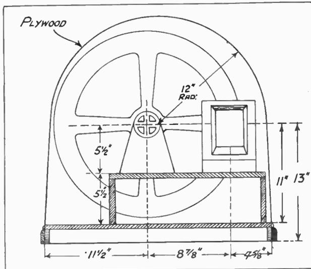
Fig. 3.—The general scheme of component lay-out, ex cabinet front.
