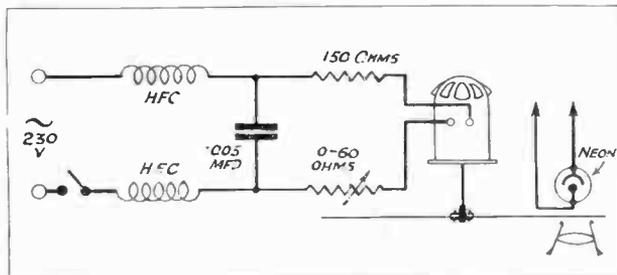
The scheme adopted for driving the motor—one which normally does duty in the home vacuum cleaner.
