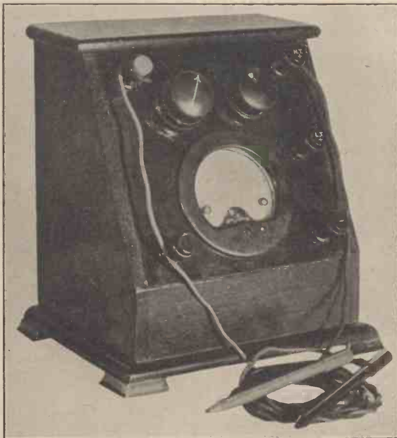
The completed "Volohmeter" is neat and very simple to use, measuring resistances and covering two ranges of voltages.
