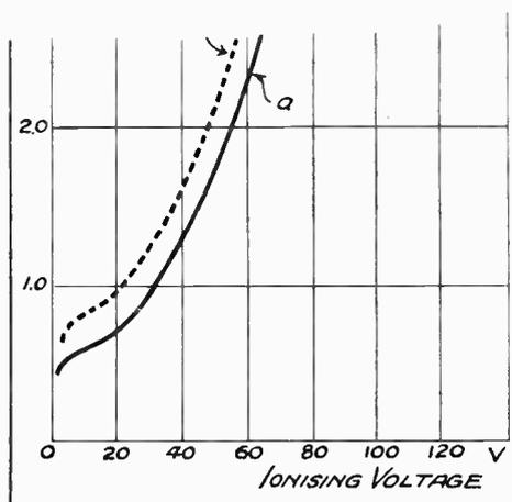
Fig. 6. Curve for potassium cell filled with argon 1.11 mm. pressure.
