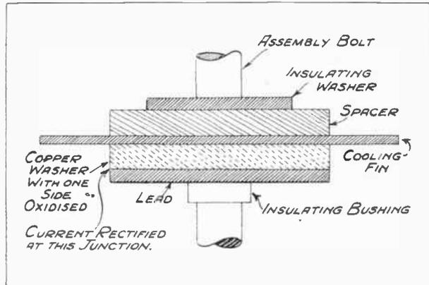
*Fig. 3.—The Westinghouse dry metal rectifier unit is built up in sections in steel bolts such as the one illustrated above.*
