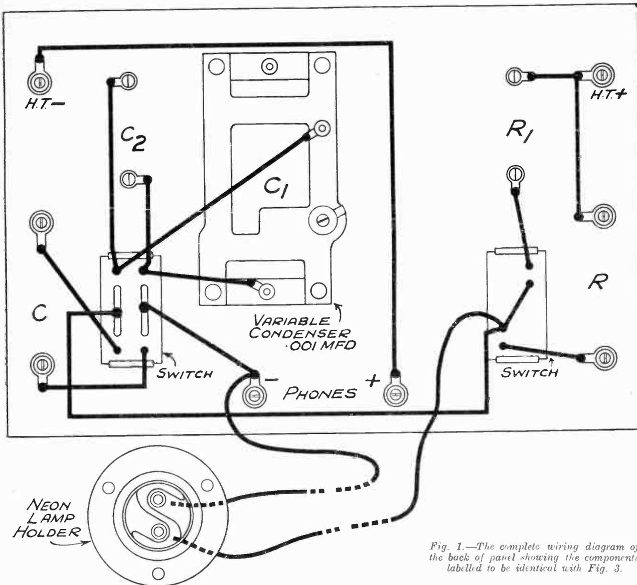
Fig. 1.—The complete wiring diagram of the back of panel showing the components labelled to be identical with Fig. 3.
