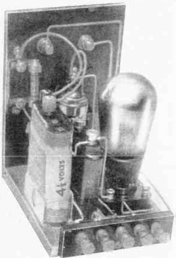
A rear view of the completed instrument showing valve and G.B. battery in position.
