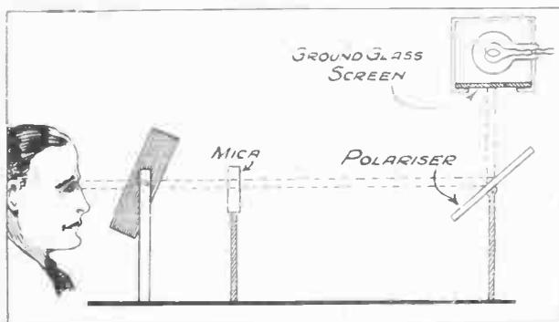
Fig. 3.—Details of a simple polariser which is very inexpensive.
