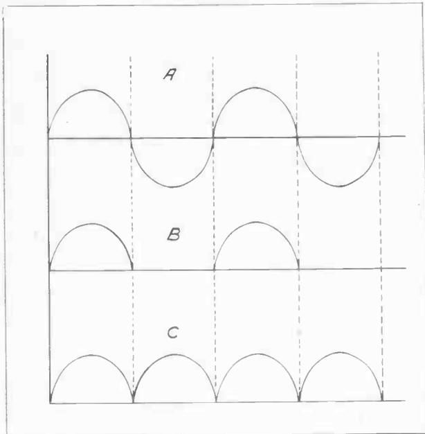
Fig. 1. Indicating alternating current at A with a half wave rectification curve at B and a full-wave rectification curve at C.
