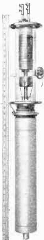
*The size of the giant Osram water-cooled valve can be gathered by a comparison with the 30" rule placed alongside*
