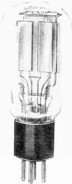
*Modern types of full-wave thermionic valve rectifiers consist of a double plate and a single filament brought out to the four pins of a standard valve base. Here we see a Mullard D.W. 30 rectifier, which is most efficient.*
