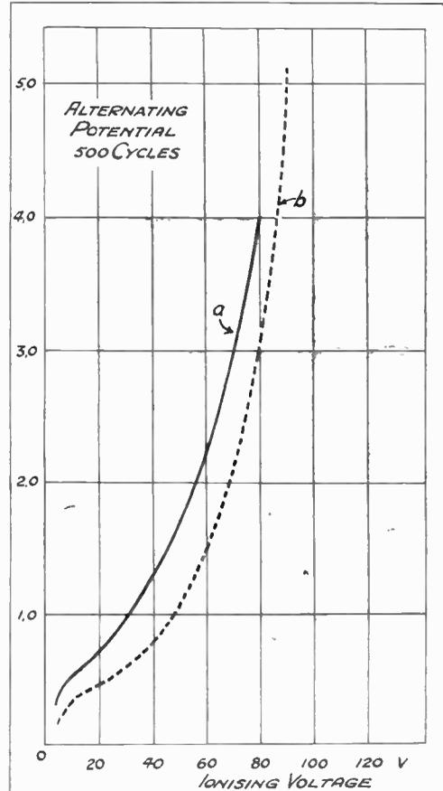
Fig. 3. Curve for potassium cell filled with neon 1.44 mm. pressure.
