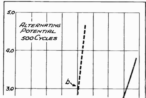
Fig. 5. Curve for potassium cell filled with helium 1.8 mm. pressure.
