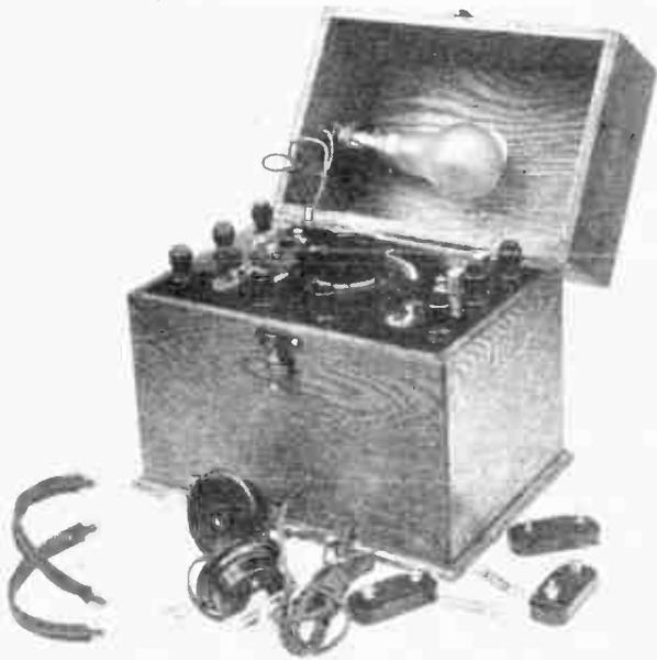
*Not how the neon lamp has been accommodated on the left-hand side of the lid. Be careful to ensure that the flexible leads do not get jammed when the lid is closed.*
