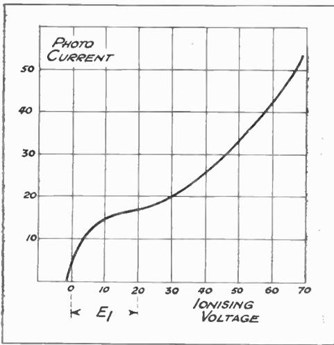
Fig. 2. Showing the behaviour of ionised gas particles (Neon-helium at 1 mm. pressure.)
