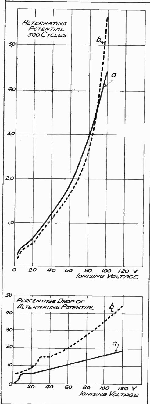
Fig. 4. Curve for potassium cell filled with helium 1.8 mm. pressure.
