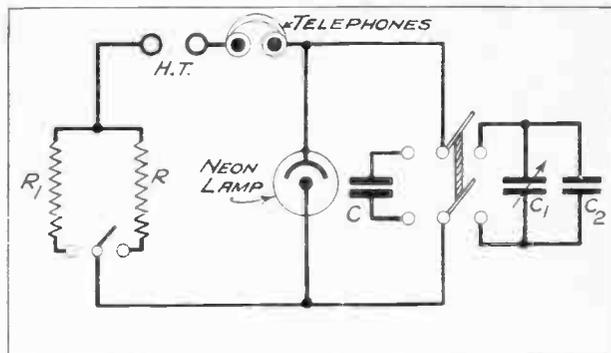
Fig. 3.—The theoretical diagram for the tester is shown here so that you can find exactly how the condensers and resistance are referred to.
