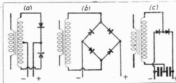
*Fig. 4.—Three methods of obtaining full-wave rectification with the dry metal unit.*
