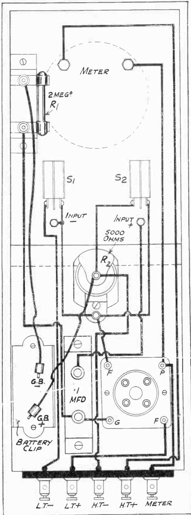
Fig. 3.—Neat and compact, little difficulty will be experienced in wiring if this diagram is followed carefully.
