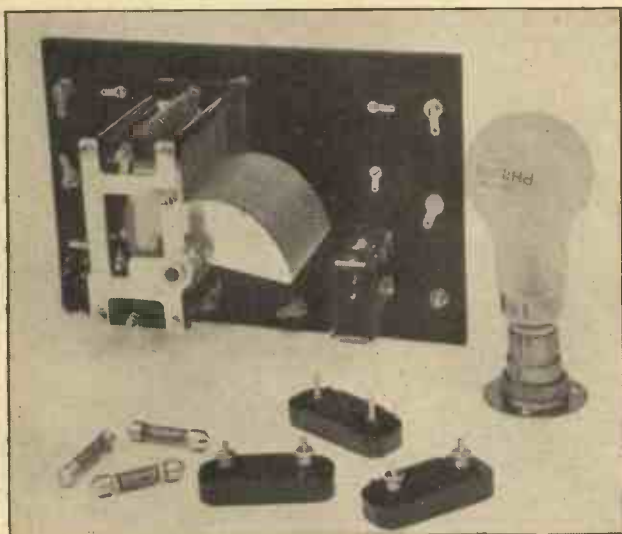
Before wiring up, the back of panel has this appearance. Note the grid leaks, condensers, and neon lamp in the foreground.
