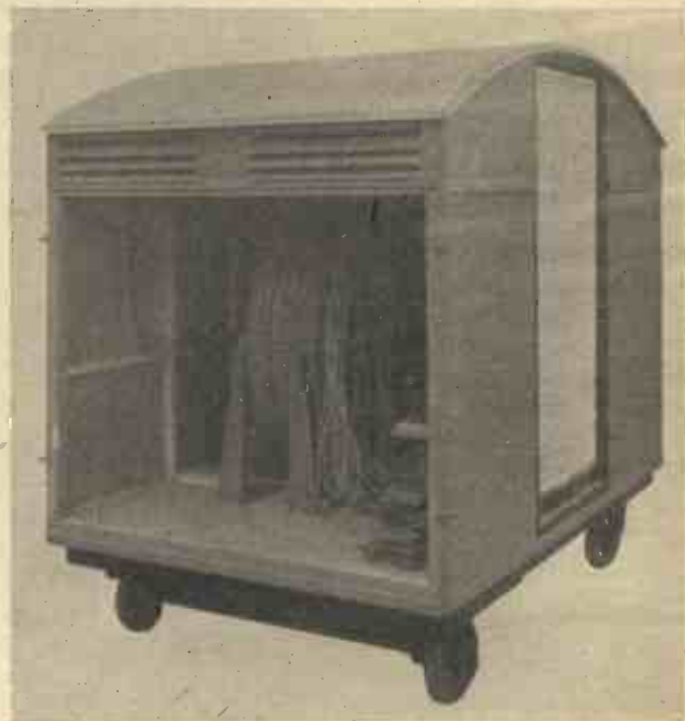
The smaller caravan made to house the Baird Lamp Screen and enable it to be more mobile than the original model.
