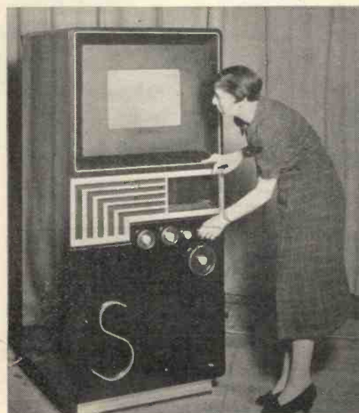
The Scophony home receiver was exhibited at last year's Radio Exhibition. The screen size was 14½ ins. X 10½ ins.
