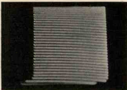
Fig. 4. Interaction between time-base circuits or too much synchronising impulse, may produce tailing of the lines.
