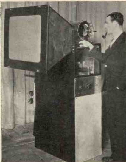
View of experimental receiver with picture 24 ins. x 22 ins., Mr. J. Sieger of the Scophony laboratories standing at the side.
