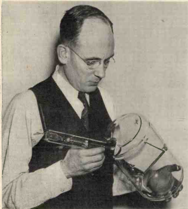
The Philco camera tube. P. J. Konkle, Philco television engineer, about to place the tube in the camera.
