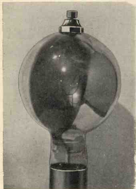
An Oxford photo-cell specially designed for television.
