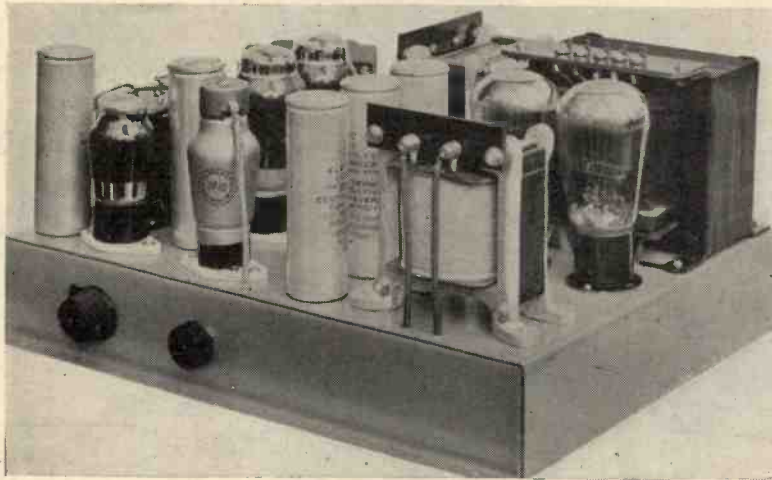
The special swinging choke is shown in the foreground of this illustration and at the left-hand side of it the smoothing condensers and Pen.-428 cathode condenser.
