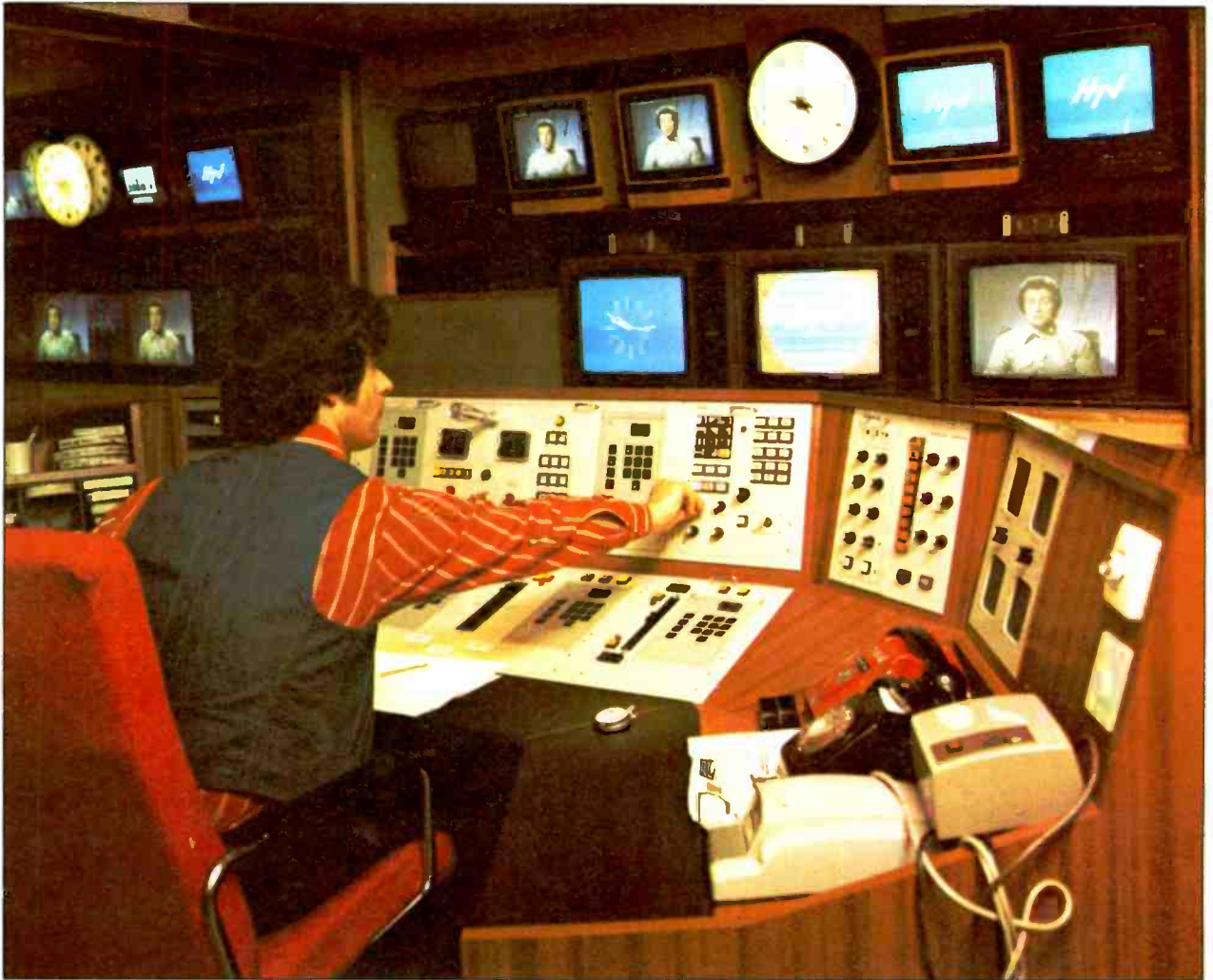
A presentation controller operates the new presentation mixer at HTV's master control in Cardiff.
