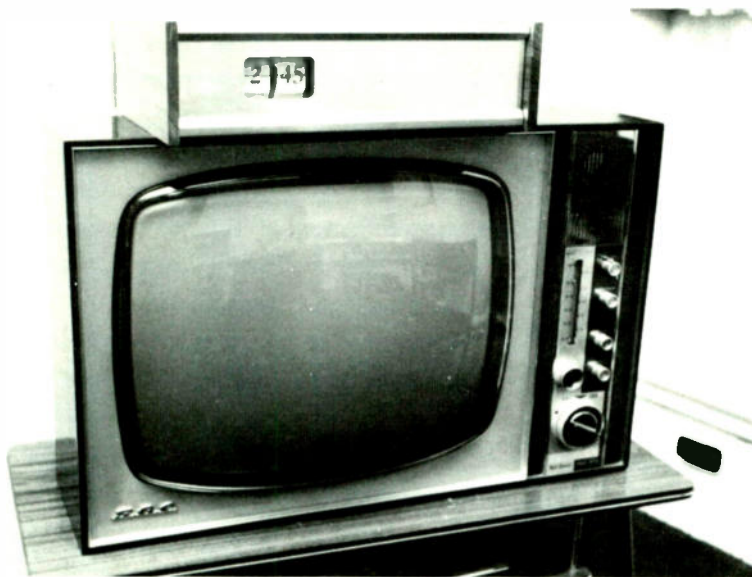
The electronic SETmeter records the amount of viewing and the channel to which viewers are tuned in 3,000 households
