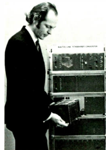
The ITA's digital lines standards converter undergoing operational testing
