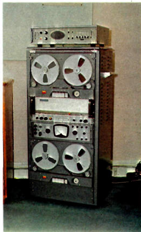
Below: Programme Services. Tape-recorder which provides a complete sound recording of the London transmitter's output for use by the Programme Services Division.
