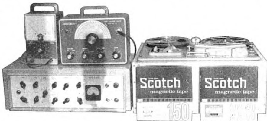
Equipment lined up for the Dynarange evaluation, including Heathkit Audio Signal Generator and Audio Valve Voltmeter, Vortexion Record/playback Amplifier and Wright & Weaire 6H Deck.
