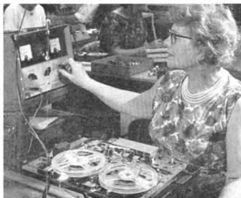
Wow and flutter check combined with speed testing.
