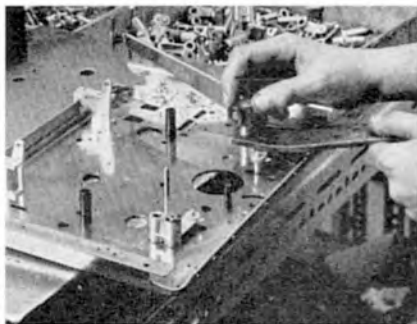
Fig. 3. Fitting and adjustment of spool carrier brackets to tape deck frame.
