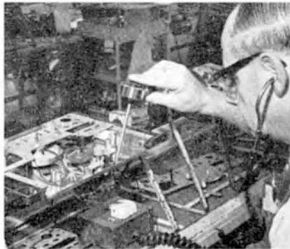
Fig. 4. Tunable stethoscope test for vibration after setting up speed change mechanism.
