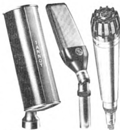
Three microphones by Tannoy. Left to right: The single element ribbon unit; Velocity ribbon microphone; and the moving coil
